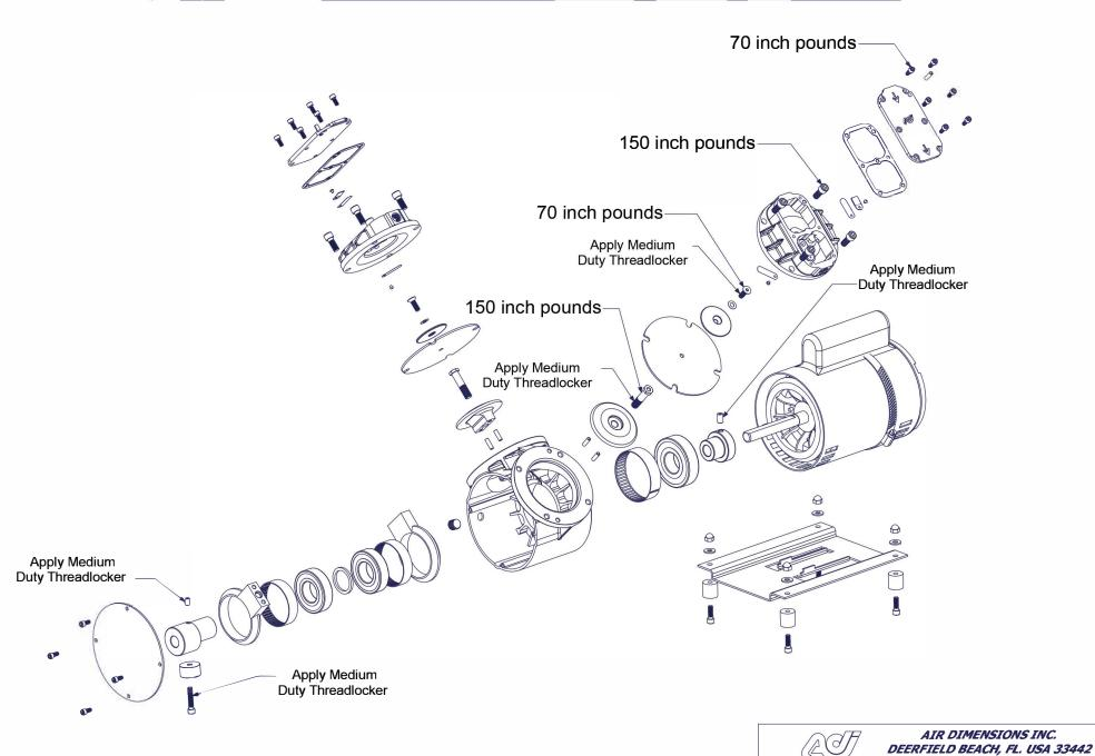
H Series Pump Torque Specs
