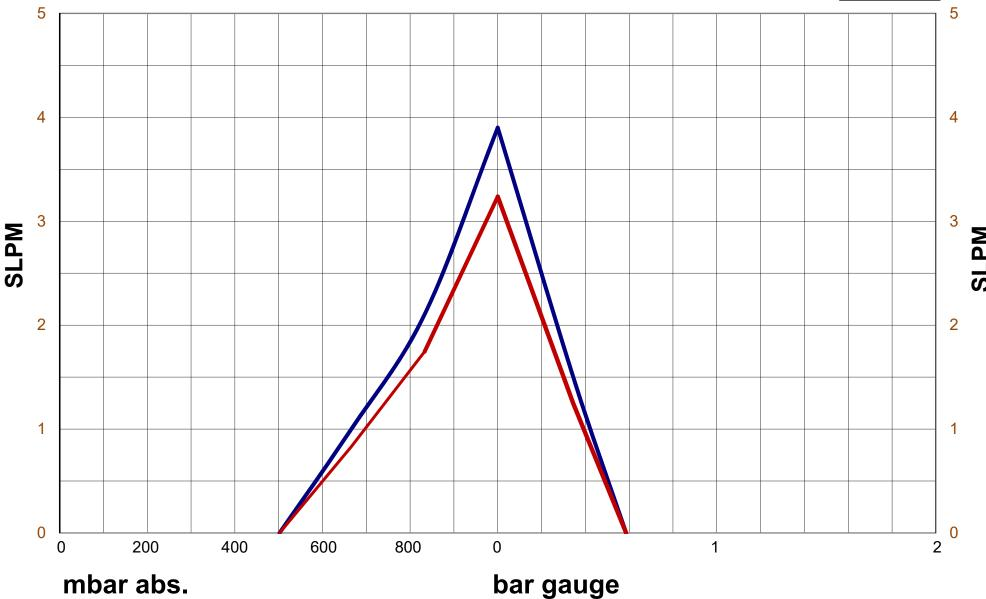
Max Pressure = 0.59 bar gauge Max Vacuum = 508 mbar abs. Max Flow = 3.9 SLPM
