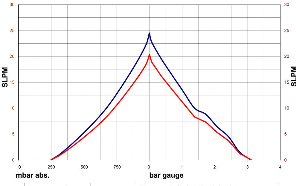
Max Pressure = 3.11 bar gauge Max Vacuum = 248 mbar abs. Max Flow = 24.5 SLPM -Test results are averaged, and therefore should be considered approximate.
