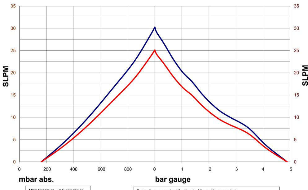
Max Pressure = 4.9 bar gauge Max Vacuum = 160 mbar abs. Max Flow = 30.25 SLPM
