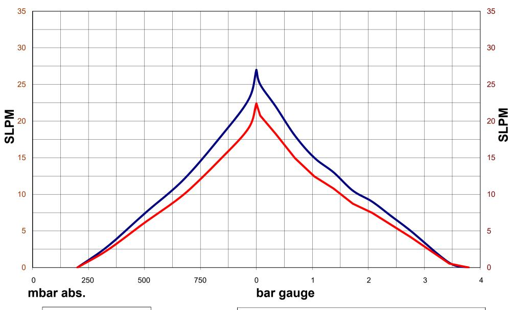
Max Pressure = 3.8 bar gauge Max Vacuum = 200 mbar abs. Max Flow = 27.0 SLPM -Test results are averaged, and therefore should be considered approximate.
