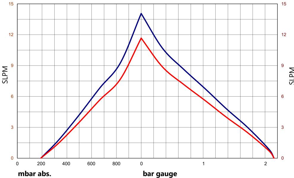
Max Pressure = 2.14 bar gauge Max Vacuum = 187 mbar abs. Max Flow = 14.0 SLPM
