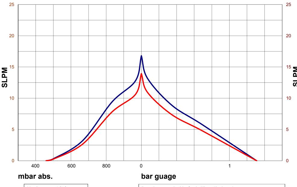
Max Pressure = 1.31 bar gauge Max Vacuum = 466 mbar abs. Max Flow = 16.8 SLPM -Test results are averaged, and therefore should be considered approximate.
